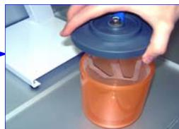
9) Holding the VMA1 push the bottom Vacuum Switch (C).
