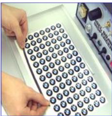
Regulable bases and superimposable dust free trays that maintains labels dust free reducing waste cost. It allows a easy level set up and a easy fix of the label sheet by using magnetic strip or profiles or by using remount spray adhesive.
